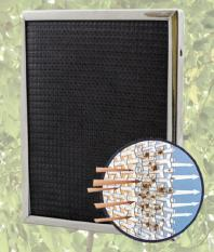
holding capacity. When particulates build up on the prefilter, air flow causes them to break off and be swept into the ACCUMULATOR CHAMBER, where turbulence and electrostatic forces cause agglomeration into even larger particulates. These agglomerated particulates are too large to pass through the second panel (afterfilter). Finally, the afterfilter attracts and holds the smaller particulates that may have escaped the prefilter, or do not respond to an electrostatic charge.
