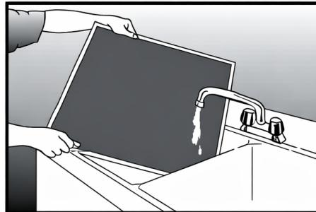
Clean monthly by rinsing DustEater with running water. Particles inside the ACCUMULATOR CHAMBER as well as on the electrostatic panels wash out easily through the drainage ports. For tough dirt and grease, use a mild detergent and rinse thoroughly with warm water.
